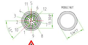
PAY ATTENTION to the position of the polarization key towards the CUT and the exagonal fixed nut.
