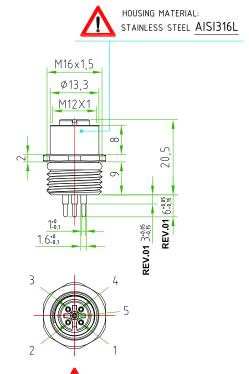
PAY ATTENTION to the position of the polarization key towards the exagonal fixing nut.
