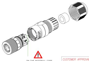
ON THE INTERNAL CORE MUST BE SILK PRINTED THE CONTACTS NUMBERS
